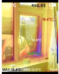
As for the mould-prone areas, this was more of a surprise. The cold area is quite clearly defined and the coldest area (11.5 °C) is where the mould has a tendency to appear. Before using the camera I thought it would show heat loss from the metal window lintel but this image suggests to me something like missing cavity-wall insulation. More investigation is required.
